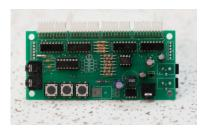
Carefully install the I/R Chip into the socket with the location notch matching the notch of the socket. The notch should be towards the two power connectors of the circuit board. The pins should be carefully aligned in the socket. Depress once aligned until fully seated on socket.
