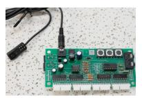
Carefully insert the Sensor into the connector until seated and secure cable.
