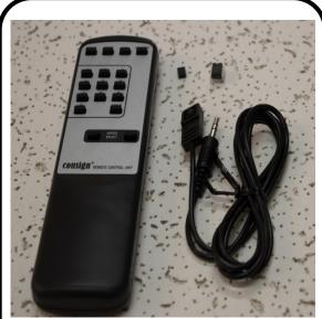
The Remote Control Kit contains the I/R Remote Contol with batteries, I/R Control Chip, I/R Sensor with 2 sided tape, and Jumper.
